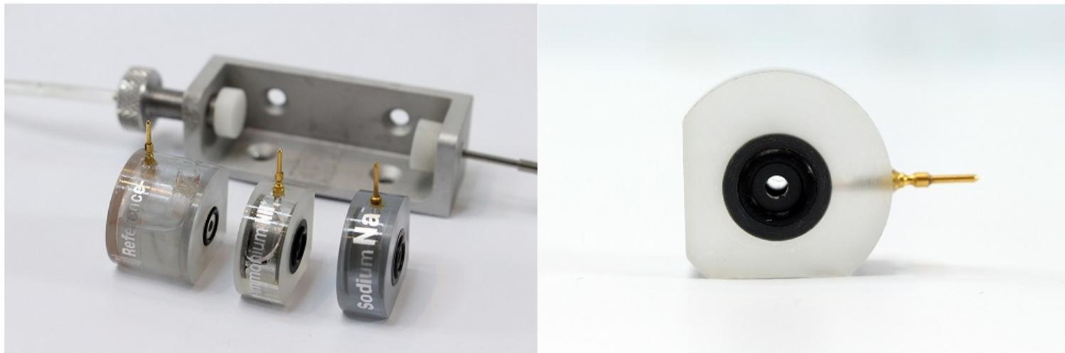
ISE Flowcells from EDT direction are solid state, zero dead volume sensors that can be used independently or positioned in series to create a multi-element sensor system. A reference flow-cell is required for each set of flow cells. The ideal flow rate is around 1-10ml per minute using a peristaltic pump. Fluoride flow-cells have an ID of 1.2mm and all the others have an ID of 2.3mm.
